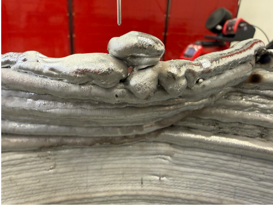
Figure 11. A deposition fault — piled / over-accumulated beads and a wall discontinuity — the class of defect 3D-registered photogrammetry is meant to detect and correct.
